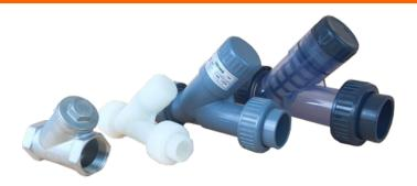
WRS Y-strainers are specially designed for chemical dosing usage. It comes with various choice of materials for different applications. Standard material shall be UPVC. User may select optional material such as CPVC, PVDF or SS304 depending on their transfer liquid. Generally, it is installed in front of a metering pump or valve to filter out solids in the liquid. It may be a small little piece of accessory, but it helps tremendously on increasing the lifespan of a dosing pump or valves.
