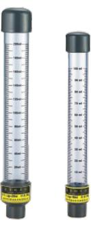
A calibration columns (also known as calibration cylinders) provide a simple method for determining pump flowrate using industry-standard graduations of milliliters/minute. All columns feature top-aligned graduated scales that allow the operator to survey in a single, one-minute test.
